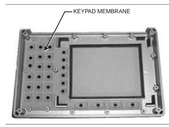
Figure 17. Front Panel Keypad Membrane
