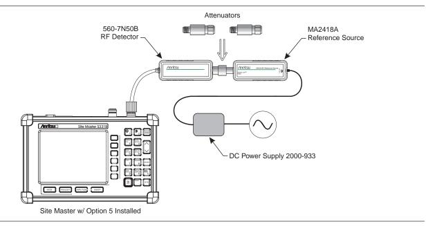
Figure 2. Power Monitor Verification
