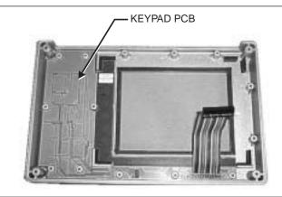
Figure 16. Front Panel Keypad PCB Location
