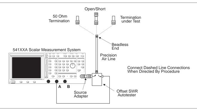
Figure 3. 541XXA Precision Return Loss Setup
