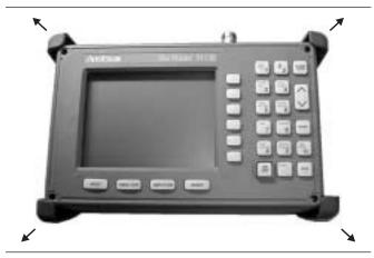
Figure 12. Removing the Corner Bumpers
