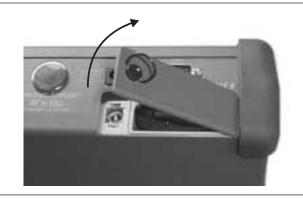
Figure 8. Removing the Battery Access Door
