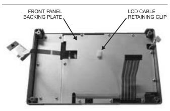
Figure 15. Front Panel Backing Plate
