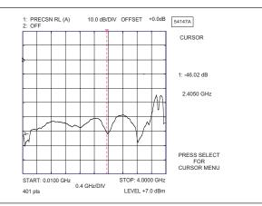
Figure 5. Direct Readout of the Precision Return Loss
