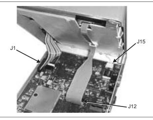
Figure 13. Site Master Front Panel Cable Connections
