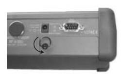
Figure 7. Rotate the Battery Access Door Handle
