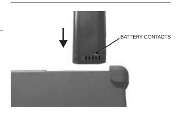
Figure 10. Battery Orientation
