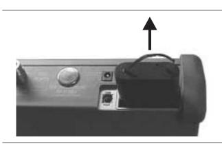
Figure 9. Removing the Battery
