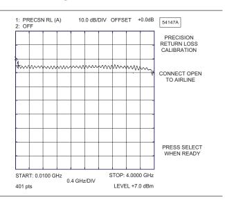
Figure 4. Example of a Good Connection
